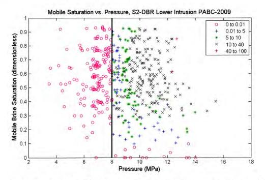
Figure 5-29: Scatter plot of mobile brine saturation versus pressure for replicate 1, S2-DBR scenario, lower drilling intrusion, all intrusion times, PABC-2009. Symbols indicate the range of DBR volumes in m<sup>3</sup>.
