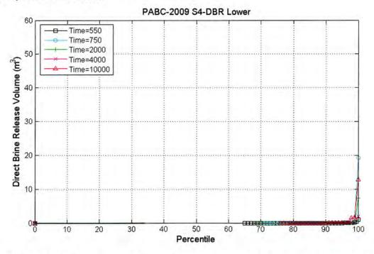
Figure 5-14: Plot of the percentile (x-axis) of DBR volumes that are less than the DBR volume on the y-axis for the PABC-2009 at the lower intrusion location for replicate 1; scenario S4-DBR.
