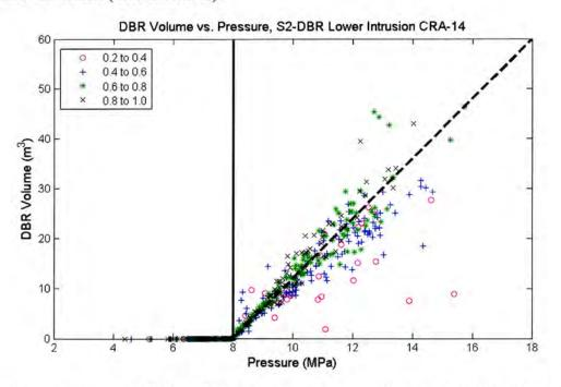
Figure 5-25: Scatter plot of DBR volume versus pressure in the intruded panel for replicate 1, S2-DBR scenario, lower drilling intrusion, CRA-2014 PA. Symbols indicate the range of mobile brine saturation (dimensionless).
