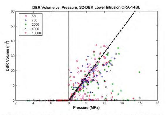
Figure 5-21: Scatter plot of DBR volume versus pressure in intruded panel for S2-DBR scenario, lower drilling intrusion, case CRA14-BL. Symbols indicate intrusion times in years.
