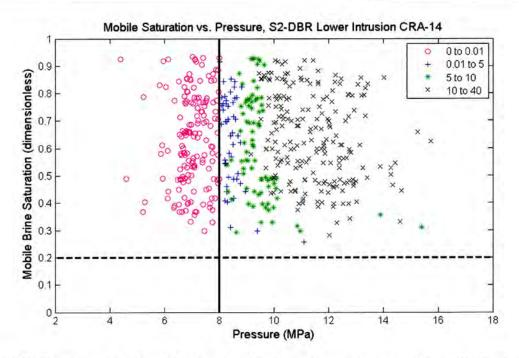
Figure 5-28: Scatter plot of mobile brine saturation versus pressure for replicate 1, S2-DBR scenario, lower drilling intrusion, all intrusion times, CRA-2014 PA. Symbols indicate the range of DBR volumes in m<sup>3</sup>.
