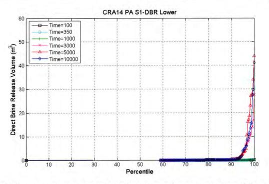
Figure 5-3: Plot of the percentile (x-axis) of DBR volumes that are less than the DBR volume on the y-axis for case CRA14-0 of the CRA-2014 PA at the lower intrusion location over all replicates; scenario S1-DBR.
