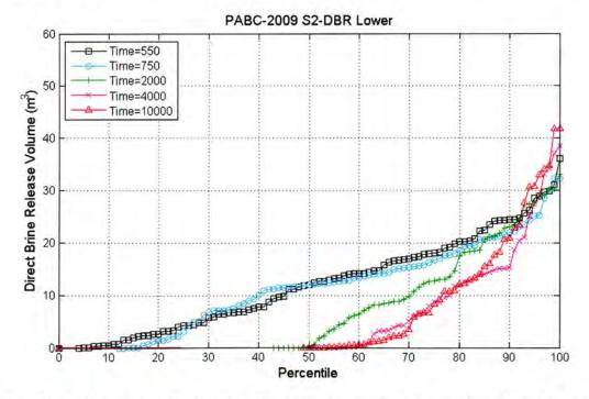
Figure 5-6: Plot of the percentile (x-axis) of DBR volumes that are less than the DBR volume on the y-axis for the PABC-2009 at the lower intrusion location for replicate 1; scenario S2-DBR.
