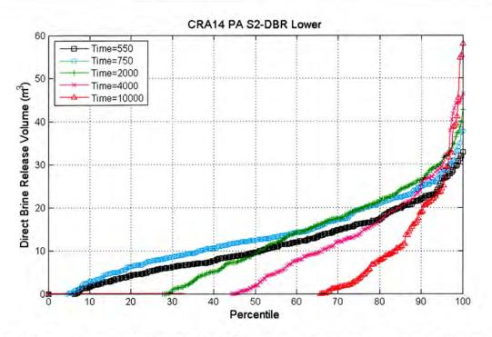
Figure 5-7: Plot of the percentile (x-axis) of DBR volumes that are less than the DBR volume on the y-axis for case CRA14-0 of the CRA-2014 PA at the lower intrusion location for all replicates; scenario S2-DBR.
