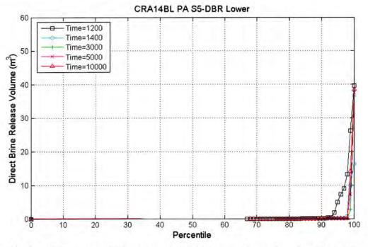
Figure 5-17: Plot of the percentile (x-axis) of DBR volumes that are less than the DBR volume on the y-axis for case CRA14-BL of the CRA-2014 PA at the lower intrusion location for replicate 1; scenario S5-DBR.
