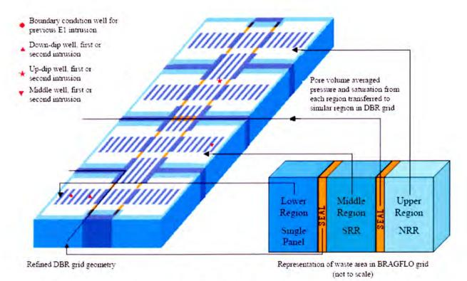
Figure 3-4. Regions to be used to transfer initial pressure and saturation from the 10,000 year BRAGFLO grid to the DBR grid for the CRA-2014.
