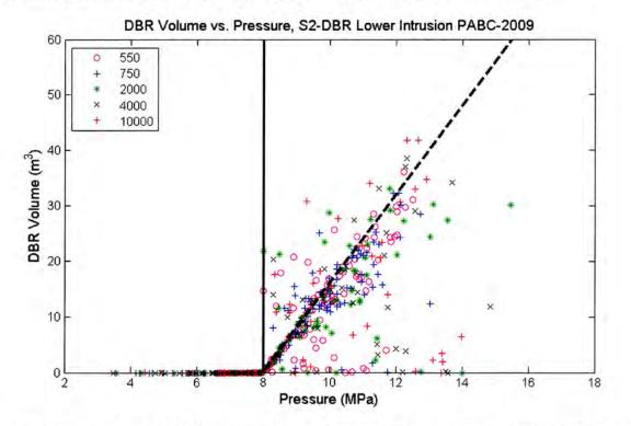
Figure 5-23: Scatter plot of DBR volume versus pressure in intruded panel for S2-DBR scenario, lower drilling intrusion, PABC-2009. Symbols indicate intrusion times in years.
