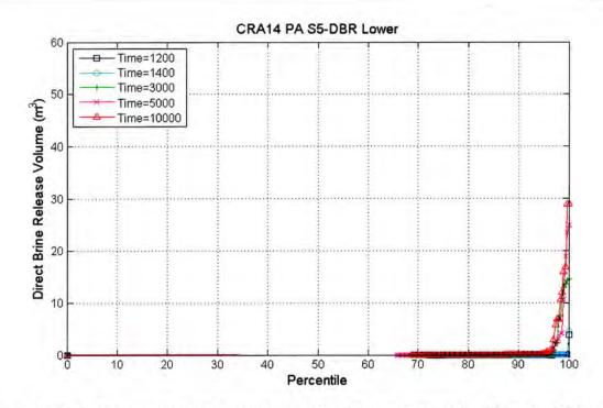
Figure 5-19: Plot of the percentile (x-axis) of DBR volumes that are less than the DBR volume on the y-axis for case CRA14-0 of the CRA-2014 PA at the lower intrusion location for all replicates; scenario S5-DBR.
