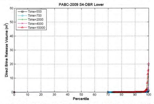
Figure 5-16: Plot of the percentile (x-axis) of DBR volumes that are less than the DBR volume on the y-axis for the PABC-2009 at the lower intrusion location for all replicates; scenario S4-DBR.
