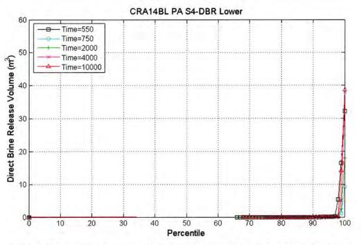
Figure 5-13: Plot of the percentile (x-axis) of DBR volumes that are less than the DBR volume on the y-axis for case CRA14-BL of the CRA-2014 PA at the lower intrusion location for replicate 1; scenario S4-DBR.
