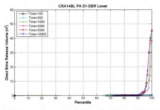
Figure 5-1: Plot of the percentile (x-axis) of DBR volumes that are less than the DBR volume on the y-axis for case CRA14-BL of the CRA-2014 PA at the lower intrusion location for replicate 1; scenario S1-DBR.
