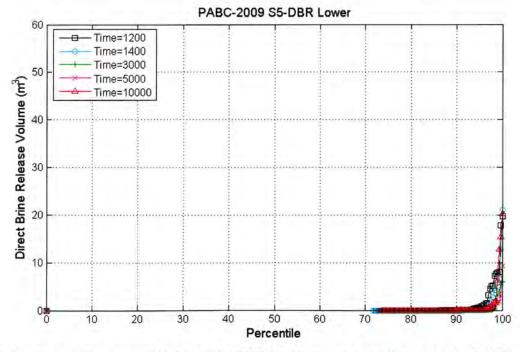
Figure 5-20: Plot of the percentile (x-axis) of DBR volumes that are less than the DBR volume on the y-axis for the PABC-2009 at the lower intrusion location for all replicates; scenario S5-DBR.
