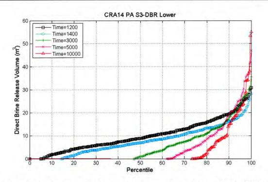
Figure 5-11: Plot of the percentile (x-axis) of DBR volumes that are less than the DBR volume on the y-axis for case CRA14-0 of the CRA-2014 PA at the lower intrusion location for all replicates; scenario S3-DBR.
