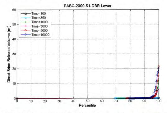
Figure 5-4: Plot of the percentile (x-axis) of DBR volumes that are less than the DBR volume on the y-axis for the PABC-2009 at the lower intrusion location for all replicates; scenario S1-DBR.
