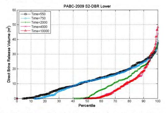
Figure 5-8: Plot of the percentile (x-axis) of DBR volumes that are less than the DBR volume on the y-axis for the PABC-2009 at the lower intrusion location for all replicates; scenario S2-DBR.
