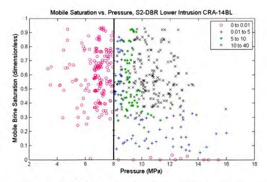
Figure 5-27: Scatter plot of mobile brine saturation versus pressure for replicate 1, S2-DBR scenario, lower drilling intrusion, all intrusion times, CRA14-BL PA. Symbols indicate the range of DBR volumes in m<sup>3</sup>.
