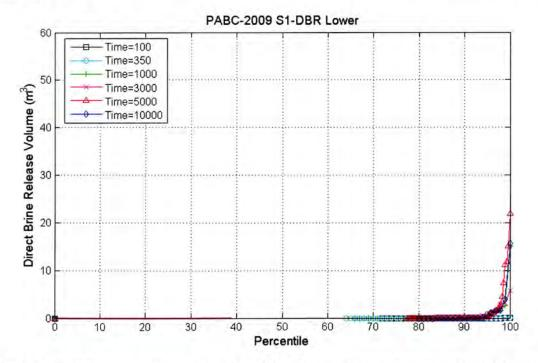
Figure 5-2: Plot of the percentile (x-axis) of DBR volumes that are less than the DBR volume on the y-axis for the PABC-2009 at the lower intrusion location for replicate 1; scenario S1-DBR.
