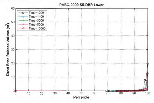
Figure 5-18: Plot of the percentile (x-axis) of DBR volumes that are less than the DBR volume on the y-axis for the PABC-2009 at the lower intrusion location for replicate 1; scenario S5-DBR.
