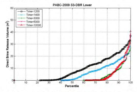
Figure 5-12: Plot of the percentile (x-axis) of DBR volumes that are less than the DBR volume on the y-axis for the PABC-2009 at the lower intrusion location for all replicates; scenario S3-DBR.
