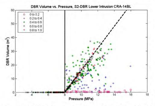
Figure 5-24: Scatter plot of DBR volume versus pressure in the intruded panel for replicate 1, S2-DBR scenario, lower drilling intrusion, CRA14-BL PA. Symbols indicate the range of mobile brine saturation (dimensionless).
