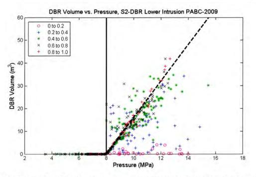
Figure 5-26: Scatter plot of DBR volume versus pressure in the intruded panel for replicate 1, S2-DBR scenario, lower drilling intrusion, PABC-2009. Symbols indicate the range of mobile brine saturation (dimensionless).
