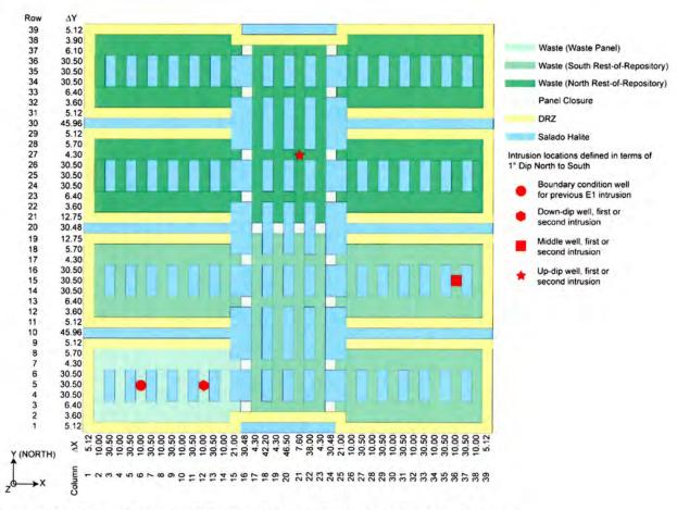
Figure 3-1: CRA-2014 PA DBR material map (logical grid) with ROMPCS.
