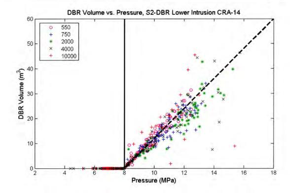
Figure 5-22: Scatter plot of DBR volume versus pressure in intruded panel for S2-DBR scenario, lower drilling intrusion, case CRA14-0. Symbols indicate intrusion times in years.
