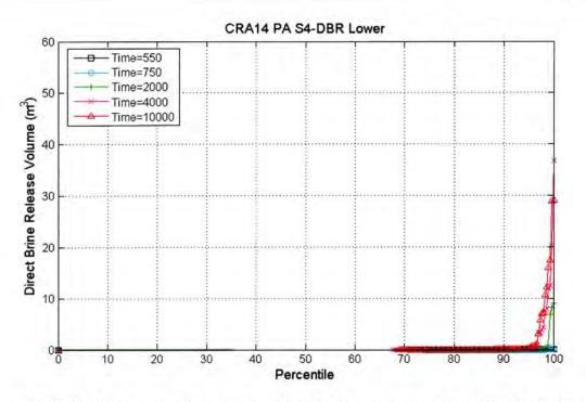
Figure 5-15: Plot of the percentile (x-axis) of DBR volumes that are less than the DBR volume on the y-axis for case CRA14-0 of the CRA-2014 PA at the lower intrusion location for all replicates; scenario S4-DBR.
